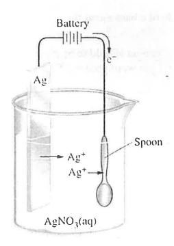
(#1) How much silver metal will be deposited on the tin spoon in 2 hours with a 5 amp current from the battery? (Silver at . wt. = 108)
